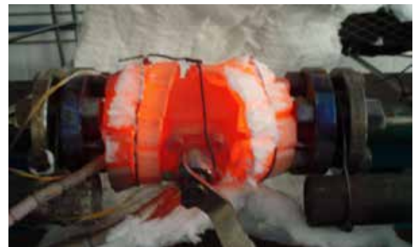
Fire safe testing of 4" - 1500 lbs
