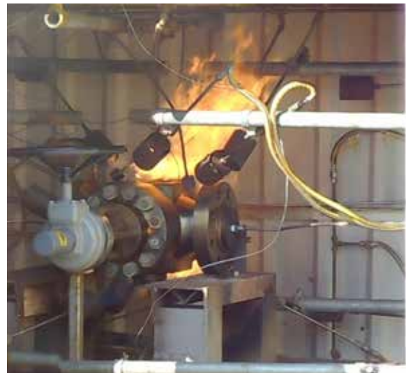
Fire safe testing of 4" - 1500 lbs
